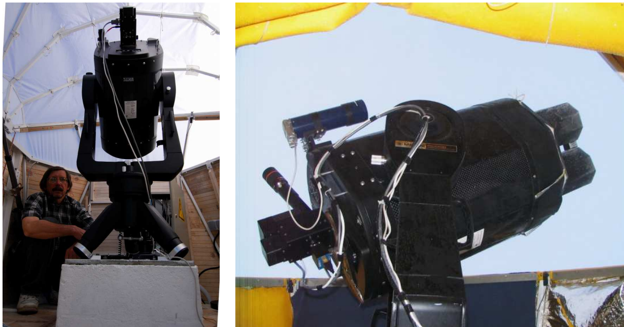
Figure 1: Telescope Meade RCX400 under the dome of automatic site testing monitor of SAI. Left: July 2007, right: March 2008
