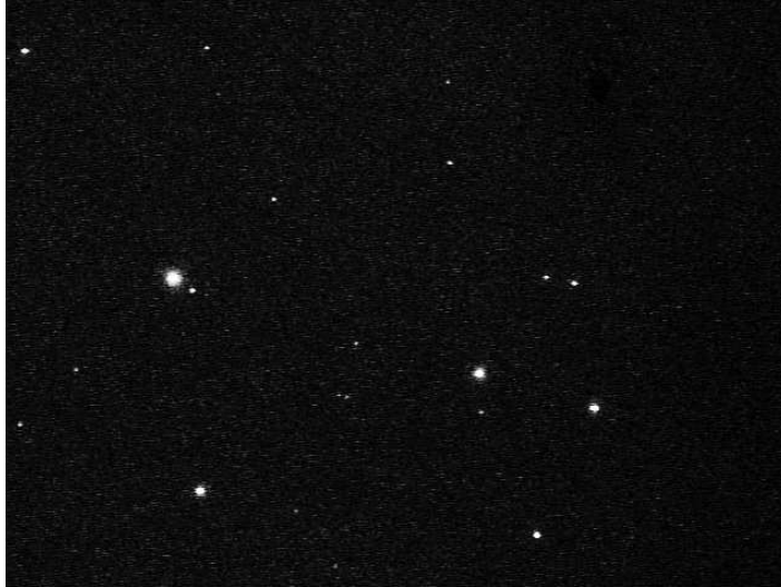
Figure 3: The Pleiades image obtained with the camera finder. The faintest star in the frame has a magnitude 8.3^m
