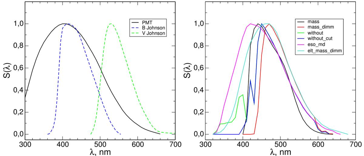
Figure 2: On the left: Photon spectral sensitivity of the PMT R7400 from Hamamatsu and the standard photometric bands  $B$  and  $V$ . On the right: The collection of the MASS spectral response curves.
