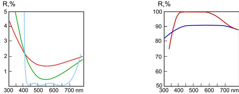
Figure 1: Reflectance of a refractive surface with AR coating (on the left). Red curve —  $\text{MgF}_2$  film on BK7 glass, green —  $\text{MgF}_2$  on SF5 glass, blue curve — enhanced multilayer coating for visual light. On the right — reflectance of Al layer without AR (blue) and with visual AR coating (red).
