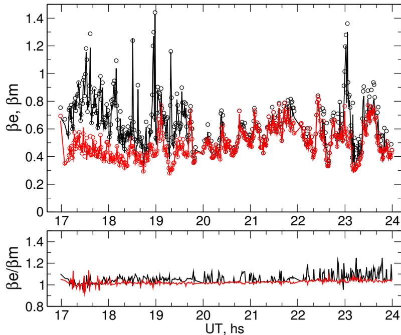
Figure 5: Upper plot: Data of the original MASS device at Maidanak for 2005-08-26. The seeing values  $\beta_E$  and  $\beta_M$  are computed from the profiles restored with the `elt_mass_dimm` (circles) and with the `mass` (line) curves, respectively. Lower plot: the ratio  $\beta_E$  to  $\beta_M$  (black — including the 0.5 km layer, red — without this layer).
